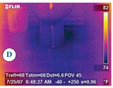
The dark spot in the infrared scan of the ceiling (B) helped to pinpoint the source of the water. Upstairs, we found that this coincided with the location of the toilet (C). As you can see in the thermal image (D), there's a darker area on right side of the toilet. A moisture meter confirmed that the floor around the toilet was soaked (E, F). We made some measurements downstairs and found that the wet
