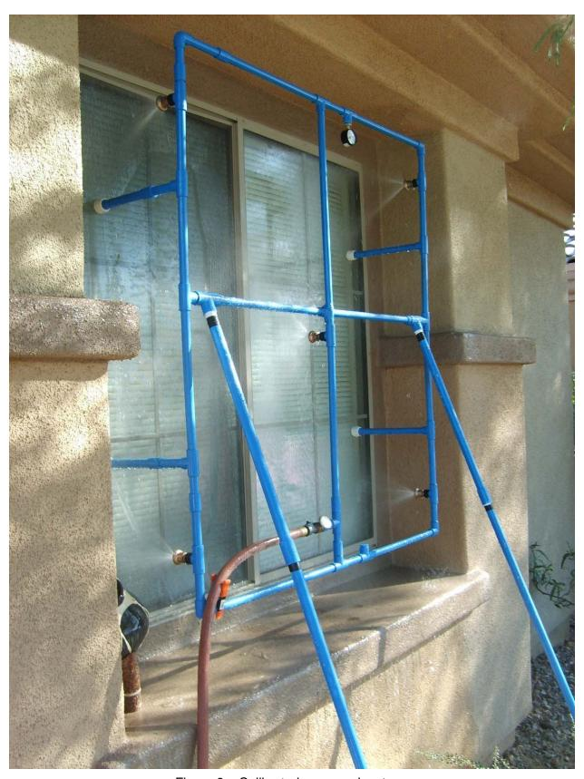
Figure 9 – Calibrated spray rack set-up.
