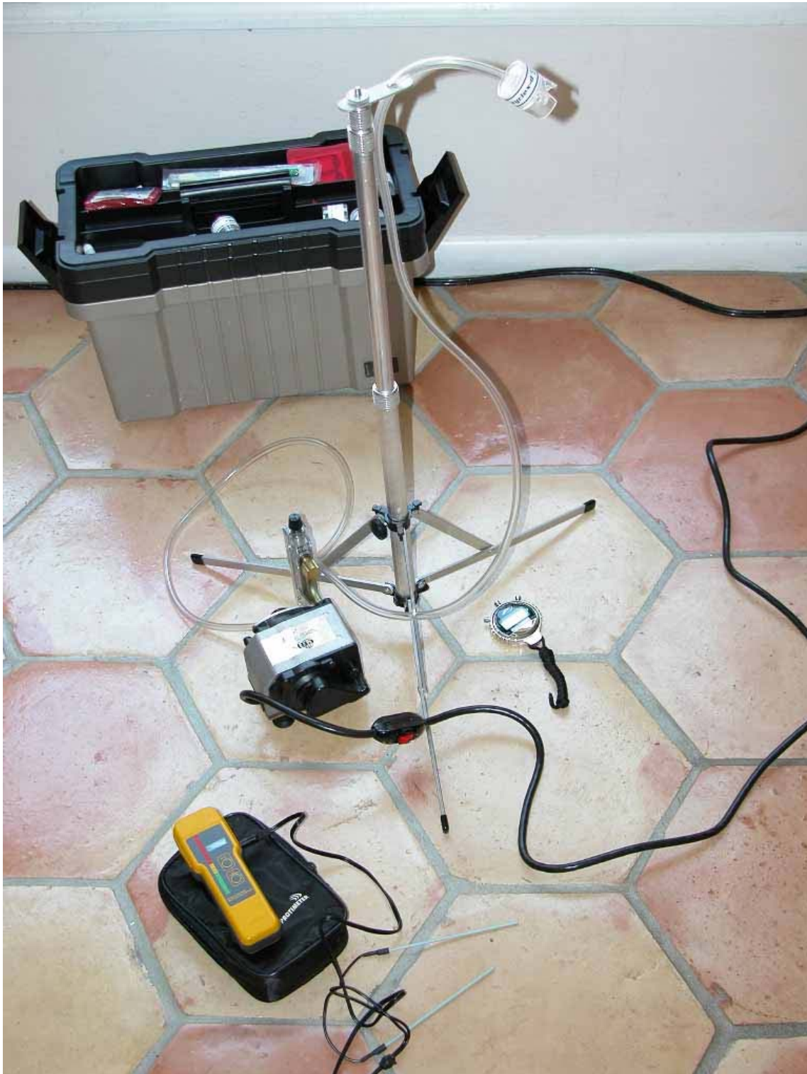
Figure 3) Vacuum pump apparatus to collect air samples
